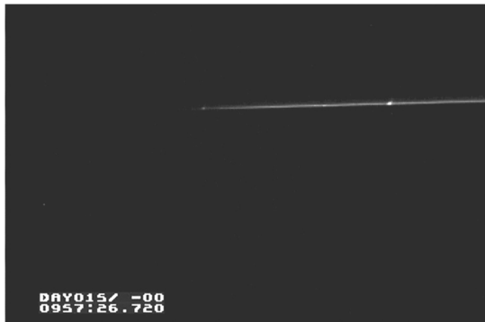
Fig. 4 A typical spectrum of the Stardust SRC's entry radiation recorded by NIRSPEC at 09:57:26.720 UT. The capsule is to the left, outside the field of view. The wavelength scale runs from left to right and is defined by the nitrogen lines at 939 (left, start of spectrum) and 1011 nm (brightest dot).
