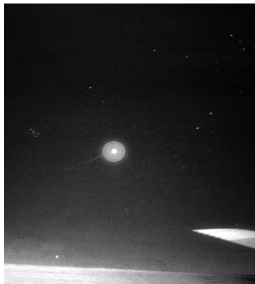
Fig. 3 The Stardust SRC entry as observed with the Xybion intensified camera.
